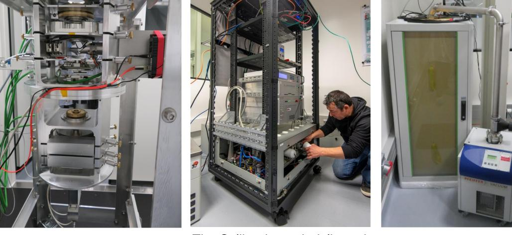
The Cassegrain unit at TBL The Calibration unit delivered by Observatoire de Hauteplane, including focal an Provence (OHP - France) achromatic polarimeter, an image stabilizing unit (ISU) and an atmospheric dispersion correction (ADC)
