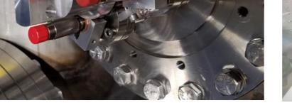
New hermetic feedthroughs (2 science + 1 reference fibers) cooled down to 2°C for thermal noise reduction
