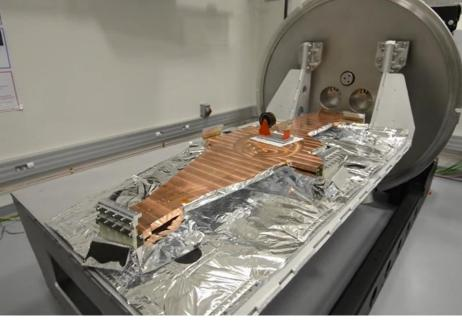
External frame and cold bus: the cold bus is linked to 2 cryocoolers.
