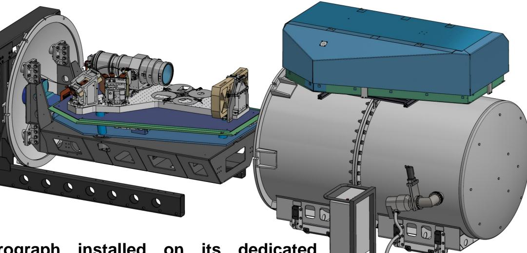
The spectrograph installed on its dedicated cryogenic bench cooled down at 70 Kelvin, within the cryostat (~ 4 m<sup>3</sup>, 10<sup>-6</sup> mbar) (initial SPIRou design: V. Reshetov (NRCH – Victoria) / improvements: E. Carrié (OMP – France)
