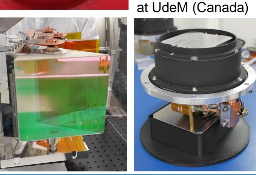
Before cooling down, the collimator is moved to its nominal position to account for the thermal shrinkage of the bench.
