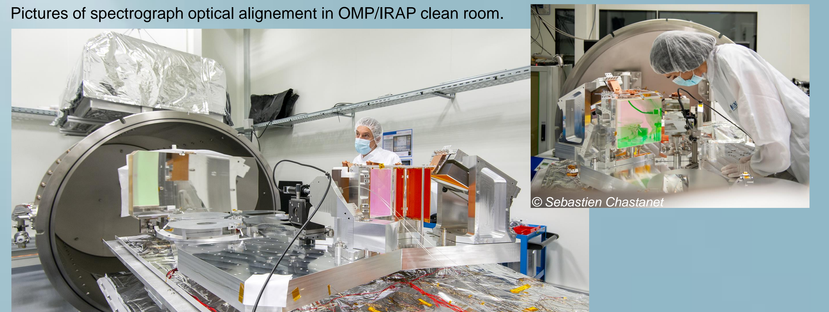
Pictures of spectrograph optical alignment in OMP/IRAP clean room.
